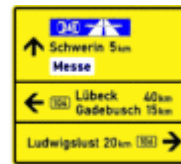
Consolidated direction sign Shows route information for all directions from the intersection
