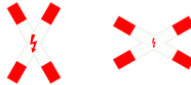
Electrified railway crossing This railroad crossing has electrical wires overhead; high profile vehicles should exercise caution
