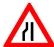
Road narrows (left side)
