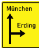
Advance direction sign Gives advance notice of directions at the upcoming intersection
