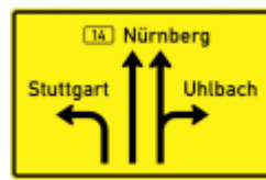
Advance direction sign Gives advance notice of directions and the lane configuration at the upcoming intersection
